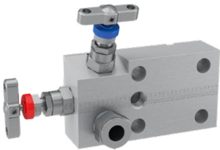
Example shown: 2-valve block and bleed direct mount manifold suitable for Emerson/Rosemount™ Coplanar™ transmitter with Parker Superior Advantage fully integrated inverted A-LOK® tube fitting connections.
